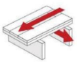
together with construction adhesive and screw into the truss/joist system every twelve inches. Additionally, nail (ring shank) or staple layers together on a minimum 12" grid pattern.
